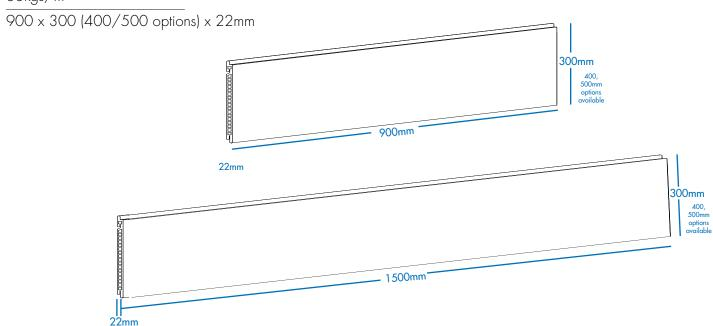
Fixing systems are available for both standard hung horizontal and vertical mounting. All panels can be produced in shorter lengths (1 mm increments)
